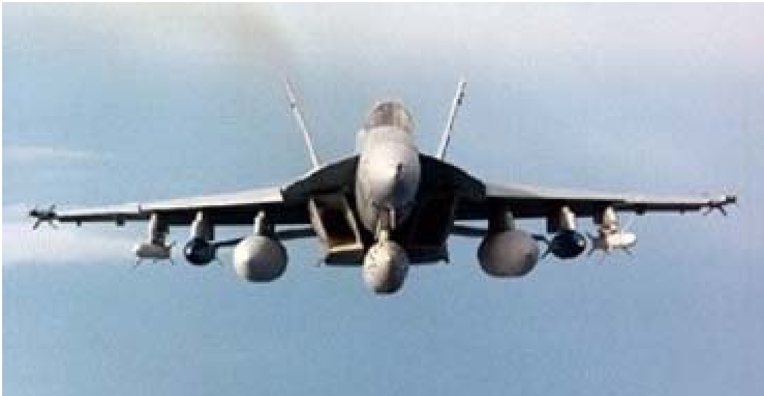
Figure 8: F/A-18E Super Hornet Illustrating 3rd Wing Pylon Store Loading
